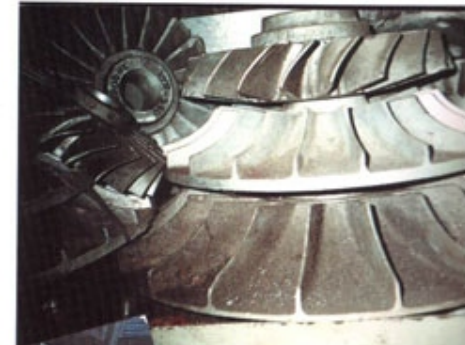
Casting of Diffuser/Blower
